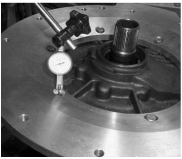
6. USING THE INDICATOR CENTER THE SPINDLE OF THE MILL OVER THE TOP OF COUNTER BORED BOLT HOLE ON THE ADAPTER PLATE.
