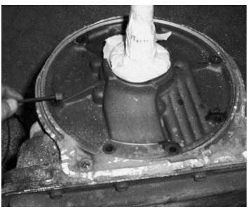
9. ONCE THE SET SCREWS ARE THREADED INTO THE CASE ABOUT 2-3 TURNS, THREAD THE  $3/8-16 \times 11/2$ " BOLTS INTO THE FRONT PUMP AND
