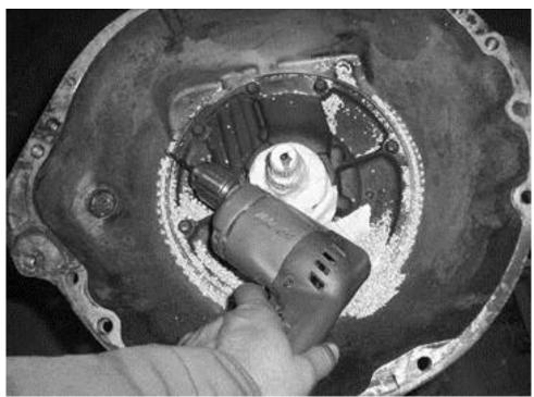
4. FROM THE BOTTOM OF THE CASE, LINED UP WITH THE EDGE OF THE OIL PAN, DRILL ACROSS THE BOTTOM OF THE CASE WITH THE 1/4" DRILL BIT.
