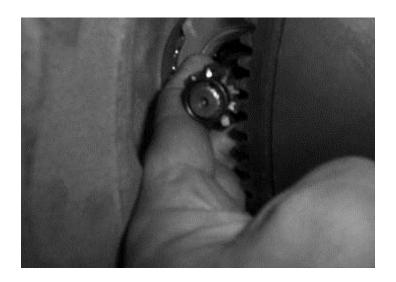
6. LUBRICATE THE NOSE OF THE TORQUE CONVERTER AND INSTALL THE TRANSMISSION TO THE ENGINE. BEFORE INSTALLING THE CONVERTER TO FLEXPLATE BOLTS, CHECK THE CLEARANCE BETWEEN THE CONVERTER AND FLEXPLATE. IT SHOULD BE BETWEEN 5/16" AND 3/16". INSTALL THE LOWER HALF OF THE BELLHOUSING AND THE REMAINING BOLTS. INSTALL THE STARTER.
