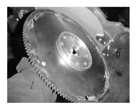
5. IT'S A GOOD IDEA AT THIS POINT TO INSTALL THE LOWER BELLHOUSING AND CHECK THE STARTER TO RING GEAR ENGAGEMENT. ONCE THIS HAS BEEN CHECKED, REMOVE THE LOWER BELLHOUSING.
